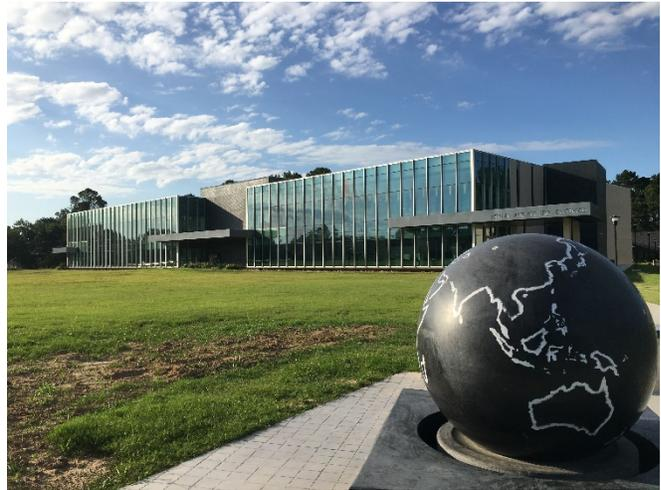
The floating granite fountain is a custom designed interactive sculpture that consists of a 5,000 pound 48” granite ball supported by a thin film of water. The granite sphere is engraved with the map of the world and engineered to rotate on the approximate axis of the Earth. As an interactive sculpture, spectators can accelerate or change the course of the floating sphere, only to have it return to its natural rotation when left alone.
